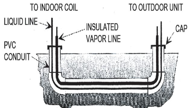
Fig.3.2 Underground Installation
